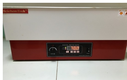
Fig 2 – Double layered heating system for heating PGC solution.
