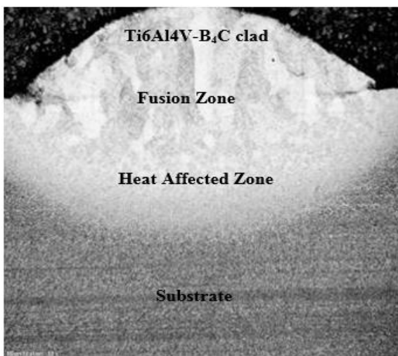
Fig. 8: Micrograph of Ti6Al4V-B 4 C composite of sample X8 at laser power of 2200 W
