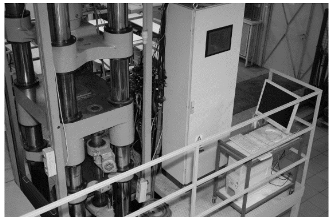
Fig. 2. Work stand for the test run of a pilot PXPh-040 press prototype
