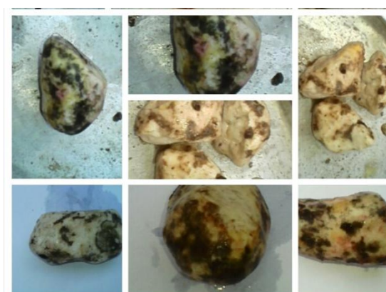
Plate 2: Physical Appearance of Plastic Samples After 23 days of Burial
