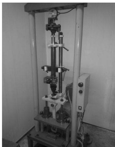
Fig. 7. Experimental stand for the shock absorber test
