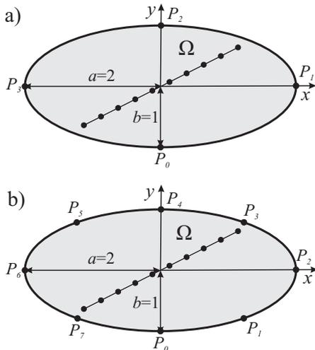
Fig. 8. Defining the shape of the boundary using a) 4, b) 8 boundary points
