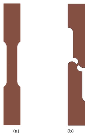
Fig. 2. Shape of the specimen; (a) Pure tension and (b) Tension+shear (combined)
