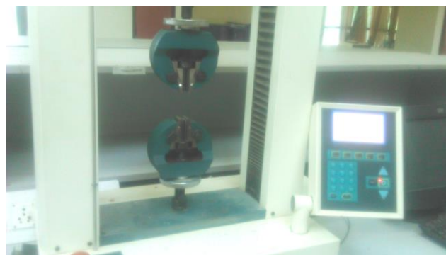
Fig. 3. Tinius Olesn H25KS tensile test machine
