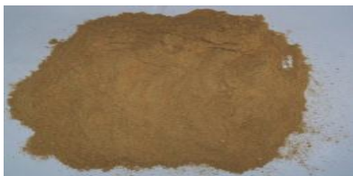
Fig. 6: Powdered ginger rhizomes with Thermal Conductivity of 0.0503W/m. K
