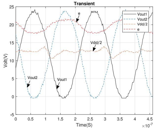
Fig. 7. Transient response of the Colpitts oscillator connected to a crystal with a resonance frequency of  $4.915MHz$
