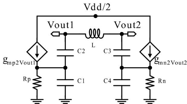
Fig. 6. Small Signal model of the CDCD Colpitts oscillator.
