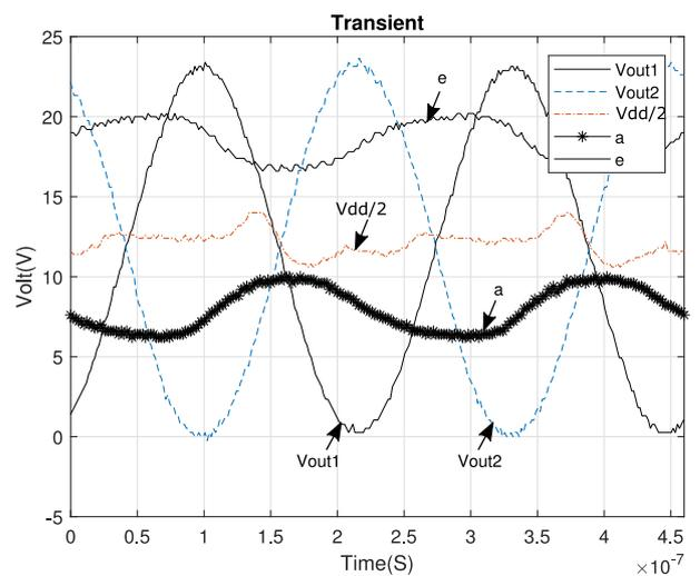
Fig. 9. Transient response of the CDCD Colpitts oscillator with an  $100\mu H$  inductor produces a frequency of ca  $4.28MHz$ .
