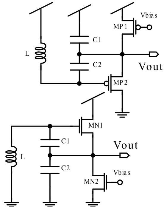
Fig. 4. Schematic of the single ended Colpitts oscillator realized using NMOS and PMOS
