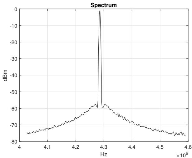
Fig. 10. Frequency spectrum of the CDCD Colpitts oscillator connected to an inductor plotted using the average function.
