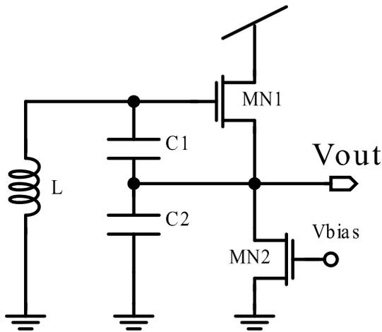
Fig. 2. A Colpitts oscillator realized using a common drain amplifier.
