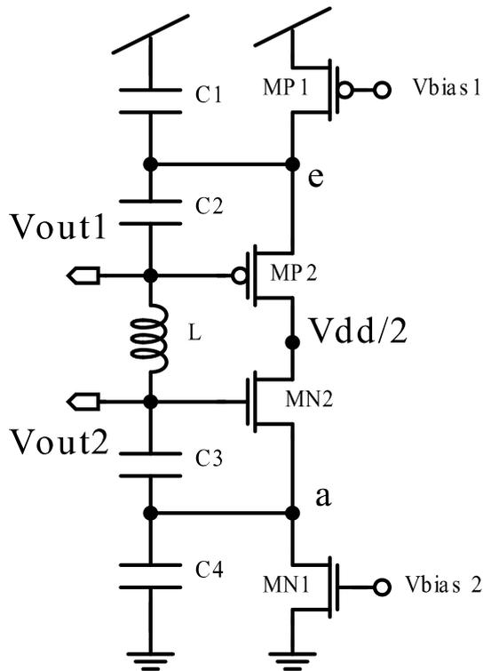
Fig. 5. Schematic of the CDCD Colpitts oscillator.
