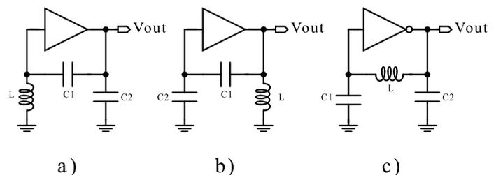
Fig. 1. Colpitts Topology, a) the inductance is connected to the input, b) the inductor is connected to the output and c) the inductor is connected between the input and the output and the amplifier needs to be inverting.
