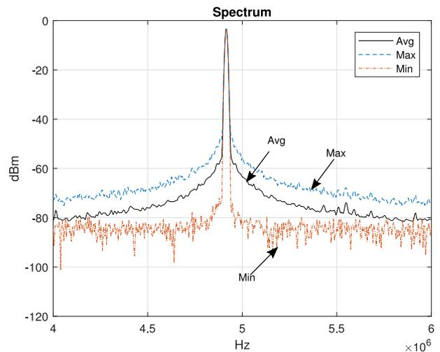
Fig. 8. Frequency spectrum of the oscillator connected to a crystal with a resonance frequency of  $4.915MHz$ .
