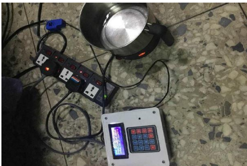
Figure 6. Measuring the Power of a Noodles Maker
