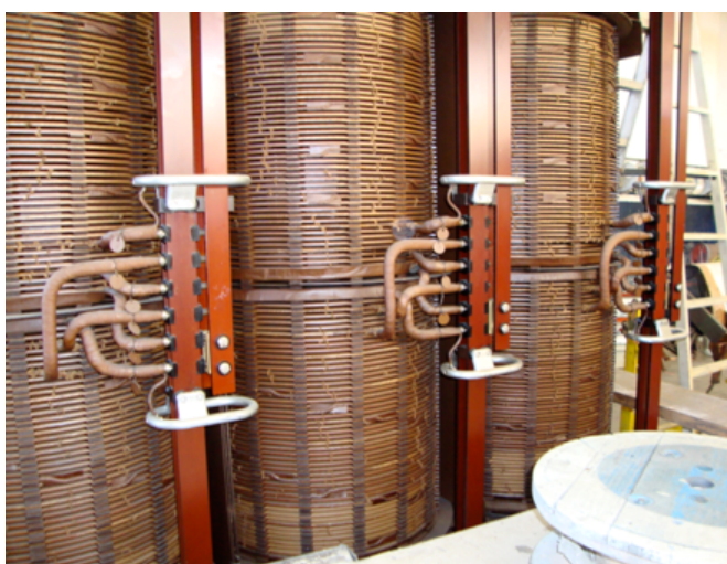
Fig. 3. Transformer primary windings
