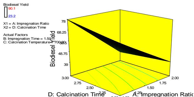
Fig. 3: A three- dimensional factorial plot for effect of impregnation ratio and calcination time on biodiesel yield
