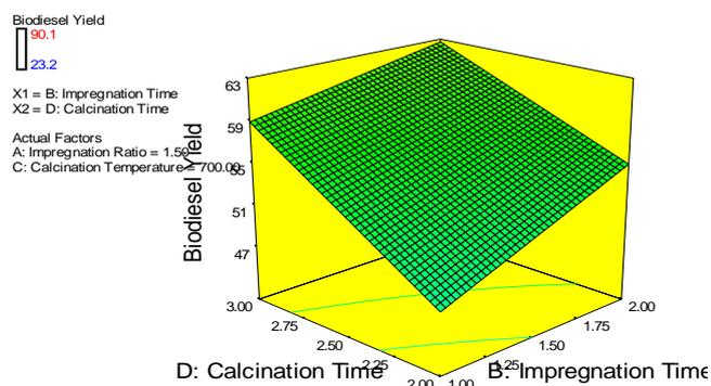
Fig. 5: A three- dimensional factorial plot for effect of impregnation time and calcination temperature on biodiesel yield
