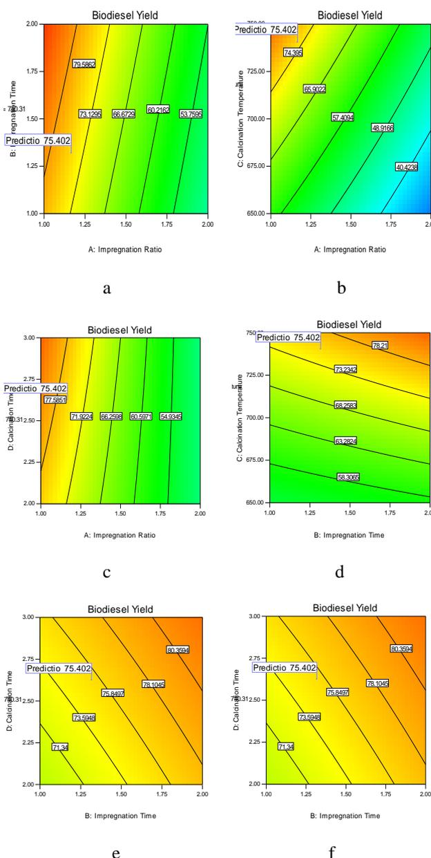
Fig. 7: Contour plots (a, b, c, d, e, & f) for the biodiesel yield predicted within the ranges of the variables studied
