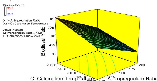
Fig. 2: A three- dimensional factorial plot on effect of impregnation ratio and calcination temperature on biodiesel yield
