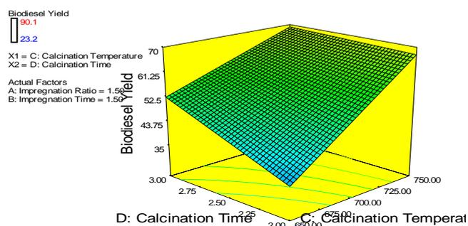
Fig. 6: A three- dimensional factorial plot for effect of calcination temperature and time on biodiesel yield
