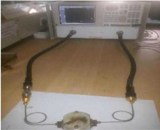
Fig. 1 Measurement set up for dielectric characterization by cavity resonator method
