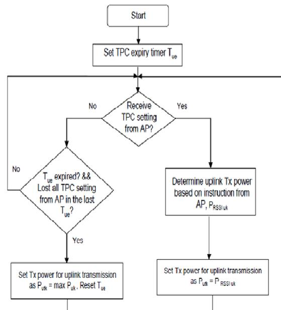
Figure 2: A flow Chart for STA TPC Mode1 operation
