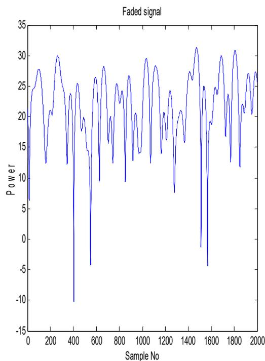
Figure 8. A simulation showing the fading effect of rain on signal power
