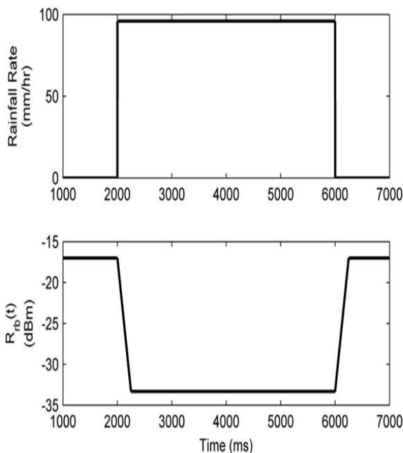
Figure 7. A plot of the system behaviour without power control in a rain event.
