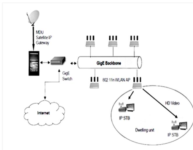
Figure 3: Typical Wireless Video Distribution System in a Multi-dwelling Unit
