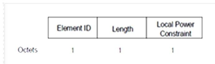
Figure 6: Power Constraint IE
