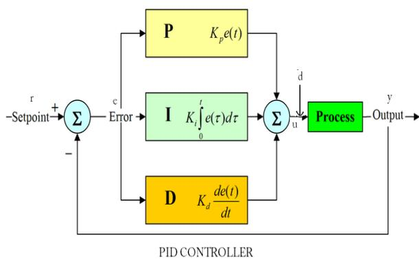
Figure 1: A block diagram showing Basic control system configuration for adaptive power control
