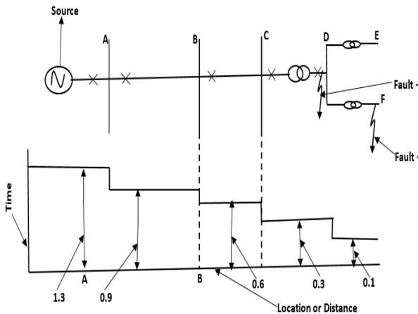
Fig. 3: Principle of a time graded over current system of protection
