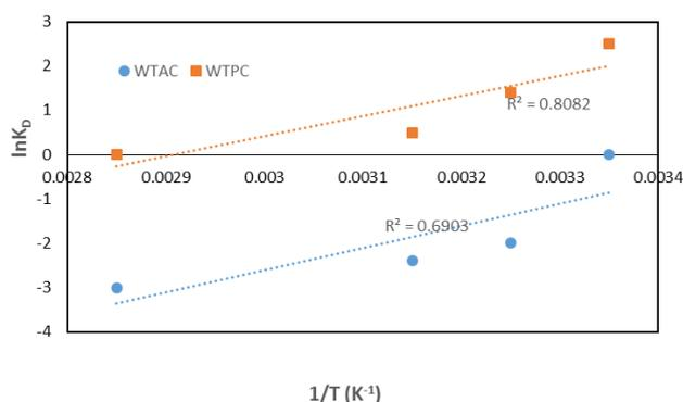
Fig. 13. Plot of  $\ln K_D$  vs  $1/T$  for the estimation of adsorption thermodynamic parameters for the adsorption of copper ions onto waste tire activated carbon
