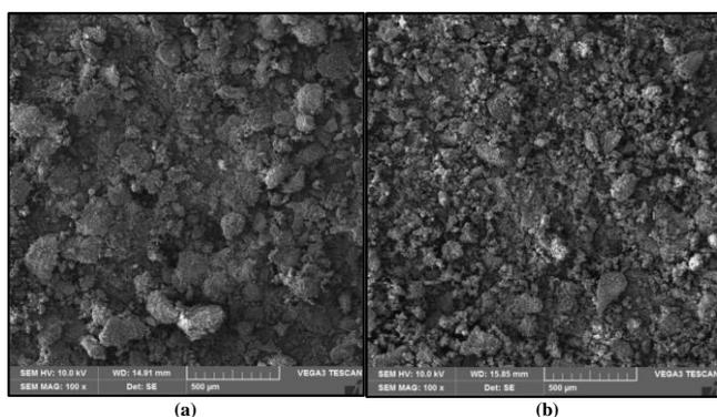
Fig. 1. SEM image of (a) waste tire pyrolysis char (WTPC) and (b) waste tire activated carbon (WTAC)
