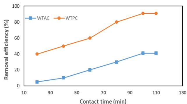
Fig. 2. Effect of contact time on the removal % of copper ions from aqueous solution (Adsorbent dosage = 0.25 g/100 mL, pH = 5, Initial metal concentration = 100 mg/L, Temperature = 25°C)
