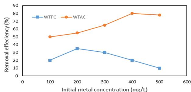
Fig. 5. Effect of initial metal concentration on the removal efficiency of copper ions from aqueous solution (pH = 5, Contact time = 100 min, Adsorbent dosage = 0.25 g/100 mL, Temperature = 25°C)
