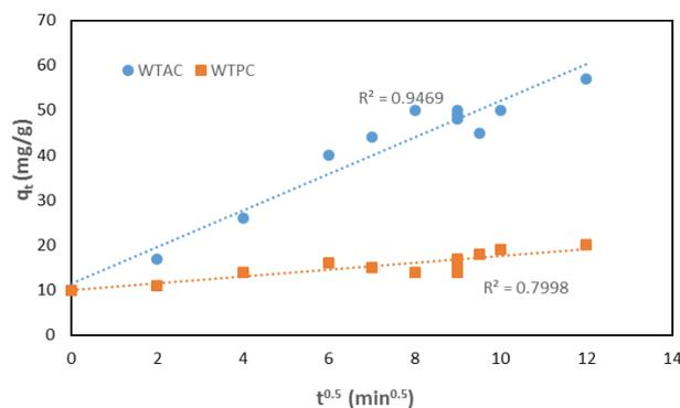
Fig. 12. Weber and Morris intraparticle diffusion kinetic model plot for the adsorption of copper ions onto waste tire activated carbon
