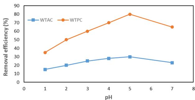
Fig. 3. Effect of pH on the removal efficiency of copper ions from aqueous solution (Adsorbent dosage = 0.25 g/100 mL, Contact time = 100 min, Initial metal concentration = 100 mg/L, Temperature = 25°C)
