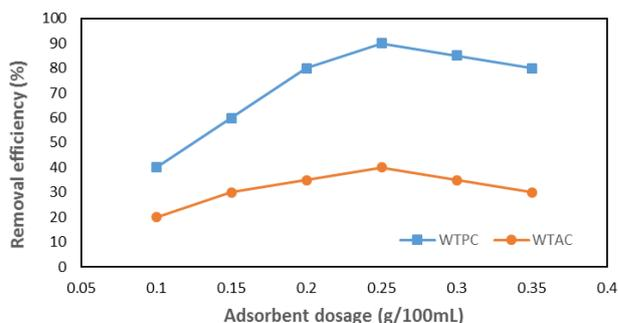
Fig. 4. Effect of adsorbent dosage on the removal efficiency of copper ions from aqueous solution (pH = 5, Contact time = 100 min, Initial metal concentration = 100 mg/L, Temperature = 25°C)
