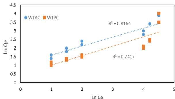
Fig. 8. Freundlich adsorption isotherm plot for the adsorption of copper ions onto WTAC and WTPC
