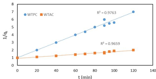
Fig. 11. Ho's pseudo-second order kinetic model plot for the adsorption of copper ions onto waste tire activated carbon
