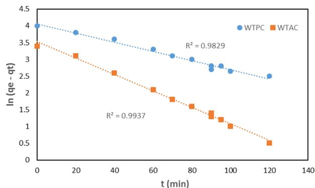
Fig. 10. Lagergren's pseudo-first order kinetic model plot for the adsorption of copper ions onto waste tire activated carbon
