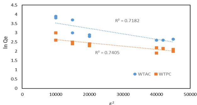
Fig. 9. Dubinin-Radushkevich adsorption isotherm plot for the adsorption of copper ions onto WTAC and WTPC
