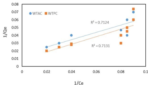
Fig. 7. Langmuir adsorption isotherm plot for the adsorption of copper ions onto WTAC and WPAC
