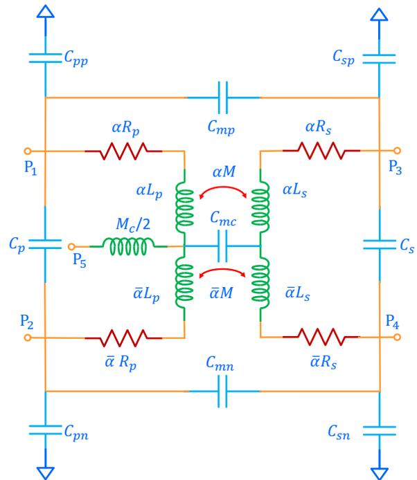
Fig. 6: Extended Balun Model with Asymmetry and More Parasitic Capacitances
