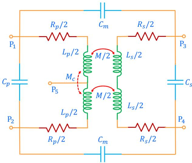
Fig. 4: Balun Model with Both Differential and Common Mode Mutual Inductance
