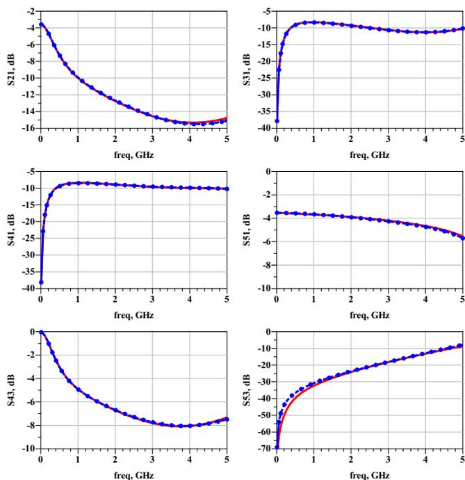
Fig. 9: Transmission. HFSS (solid) v.s. lumped (dotted).
