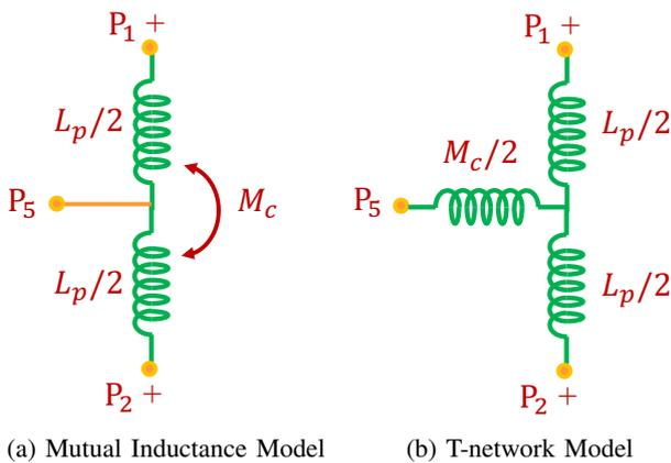
Fig. 5: Common Mode Equivalent Circuit
