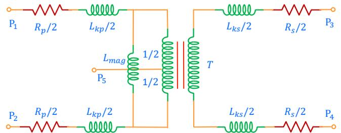
Fig. 2: Compact Balun Model Based on Ideal Transformers
