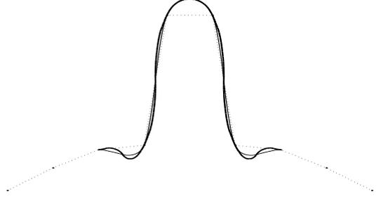
Figure 1: Open curves produced by the 4-point ternary interpolatory scheme. The thin solid line is produced by setting  $\mu = \frac{1}{11}$  and the bold solid line is produced by setting  $\mu = \frac{1}{4}$ .
