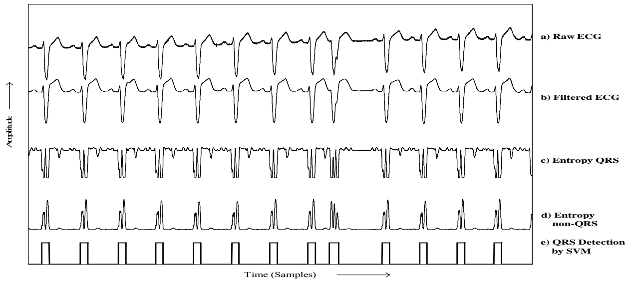
Fig.3 QRS detection of lead L 2 for record MO1_026 of CSE ECG database
