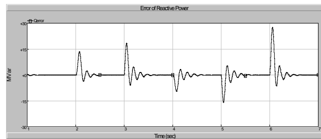
Fig. 18. (b) The calculated control error of reactive power using conventional PI controllers.
