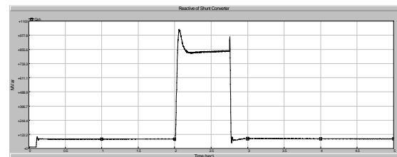
Fig. 11. The changes of output reactive power of the VSUPFC (double shunt converters).
