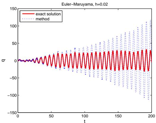
Fig. 3. A Sample Trajectory arising from the Euler-Maruyama Method (30) (blue dotted) and the True Solution (10) (red solid)
