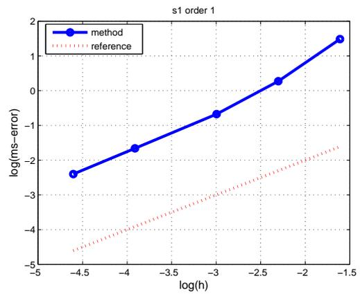
Fig. 7. Logarithm of the Mean-Square Error at Time  $t = 200$  by the Numerical Method (8), versus the Logarithm of the time step-size  $h$ , for  $h=0.01, 0.02, 0.05, 0.1, 0.2$  (blue solid), and the Reference Line of Slope 1 (red dotted)
