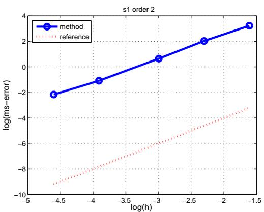
Fig. 8. Logarithm of the Mean-Square Error at Time  $t = 200$  by the Numerical Method (9), versus the Logarithm of the time step-size  $h$ , for  $h=0.01, 0.02, 0.05, 0.1, 0.2$  (blue solid), and the Reference Line of Slope 2 (red dotted)
