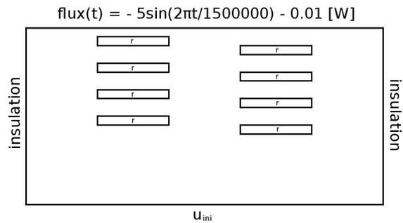
Fig. 4. The initial conditions and the thermal boundary conditions.
