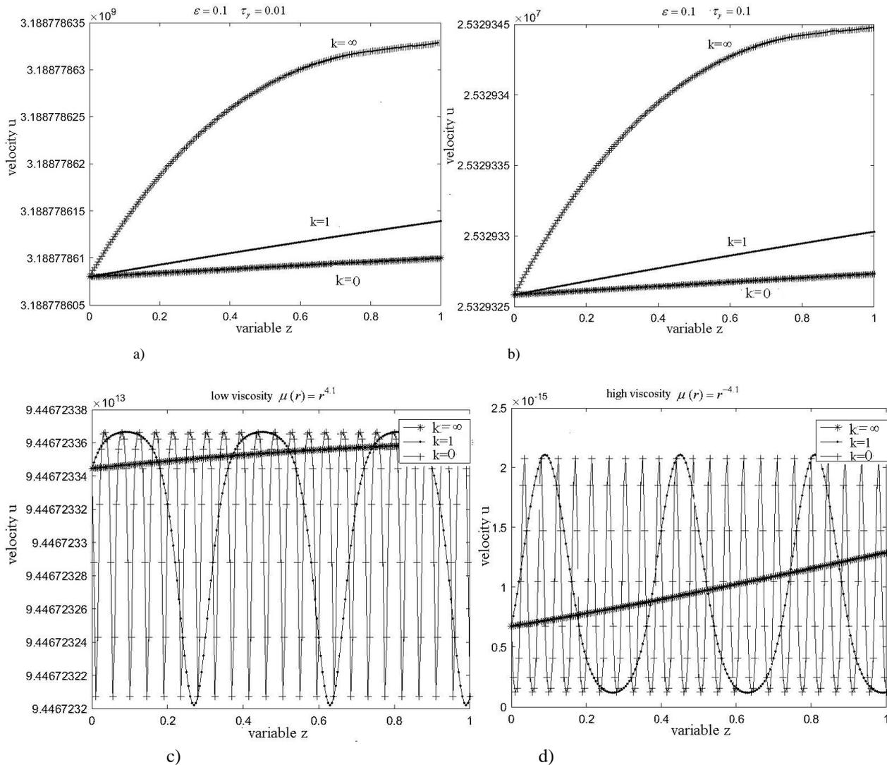
Fig. 3. Comparison of velocity profiles for different types of roughness at several values of yield stress and viscosity
