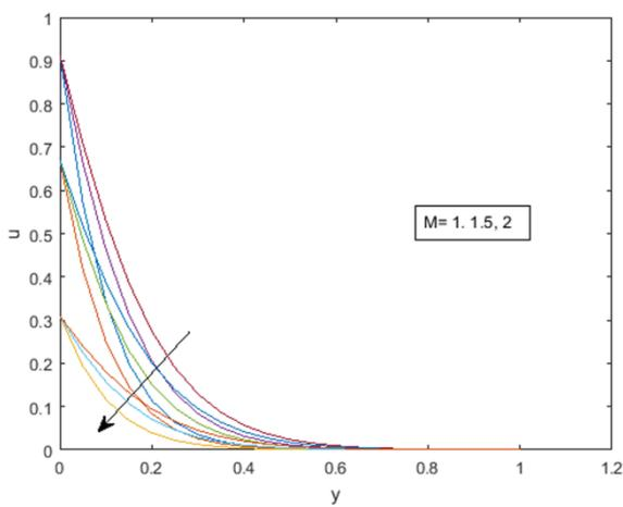
Fig 4: Effects of  $M$  on velocity Profile
