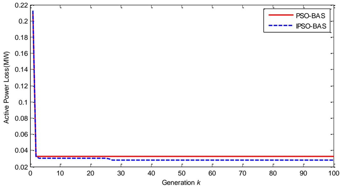
Fig.14 The active power loss convergence curves using IPSO-BAS and PSO-BAS on the IEEE 33-bus distribution network (0.866 leading power factor)
