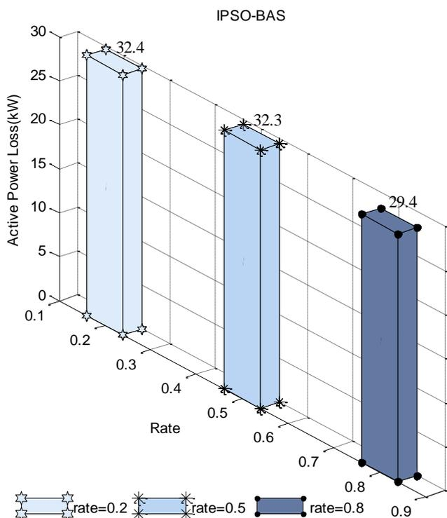
Fig.4 Active power loss using different rate for IPSO-BAS on the IEEE 33-bus system
