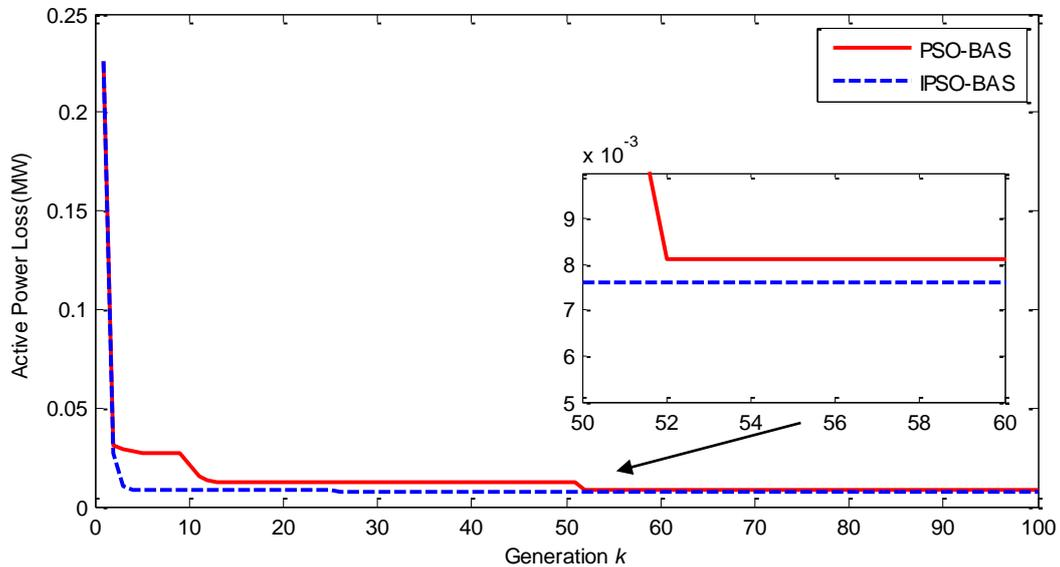
Fig.29 The active power loss convergence curves using IPSO-BAS and PSO-BAS on the IEEE 69-bus distribution network (0.866 leading power factor)
