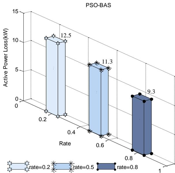
Fig.16 Active power loss using different rate for PSO-BAS on the IEEE 69-bus system
