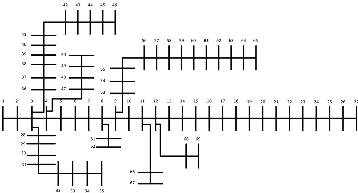
Fig.26 The schematic diagram of IEEE 69-bus radial distribution system.
