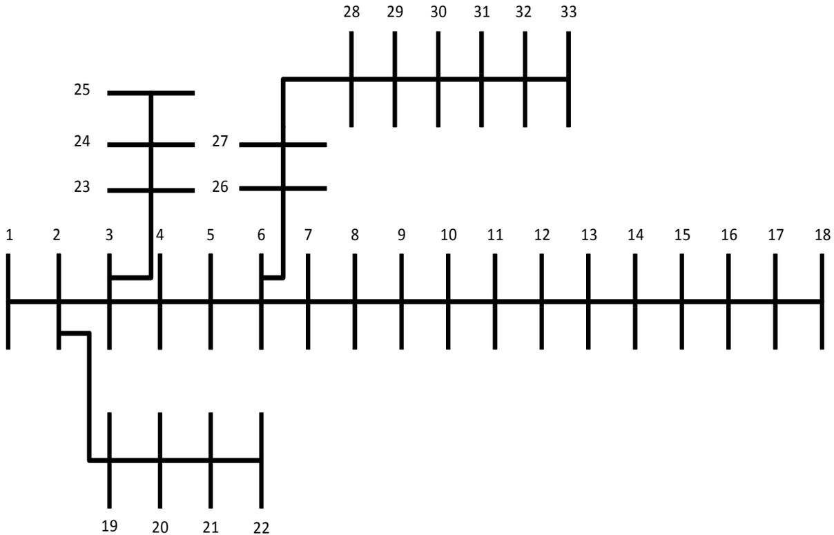
Fig.24 The schematic diagram of IEEE 33-bus radial distribution system.
