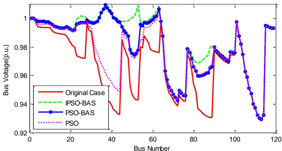
Fig.30 The node voltages for different algorithms and origin case on the IEEE 119-bus distribution network (0.866 leading power factor)
