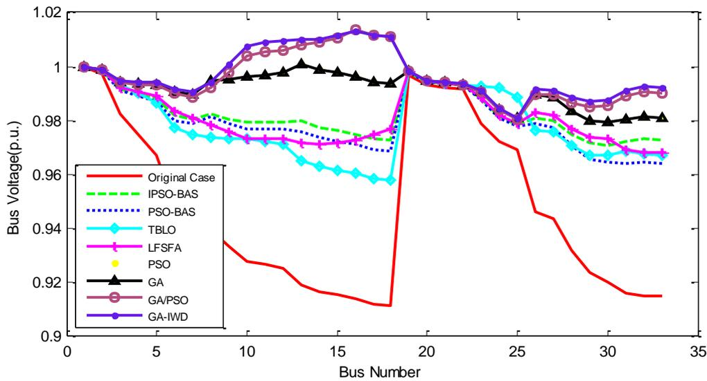
Fig.12 The node voltages for different algorithms and origin case on the IEEE 33-bus distribution network (unity power factor)
