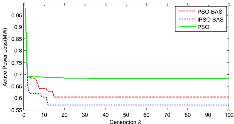
Fig.31 The active power loss convergence curves using PSO, IPSO-BAS and PSO-BAS on the IEEE 119-bus distribution network (0.866 leading power factor)
