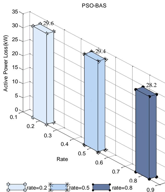
Fig.5 Active power loss using different rate for PSO-BAS on the IEEE 33-bus system
