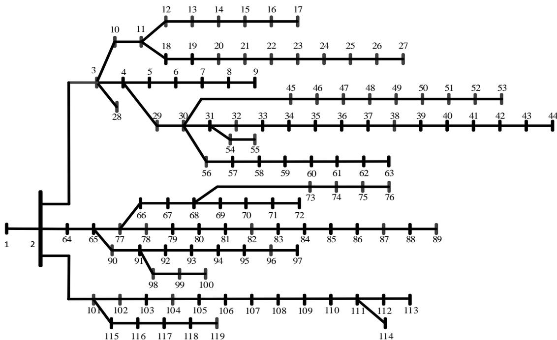
Fig.25 The schematic diagram of IEEE 119-bus radial distribution system
