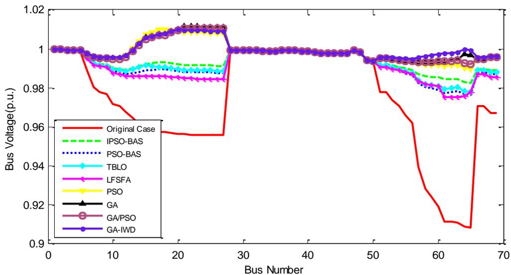
Fig.27 The node voltage for different algorithms and origin case on the IEEE 69-bus distribution network (unity power factor)
