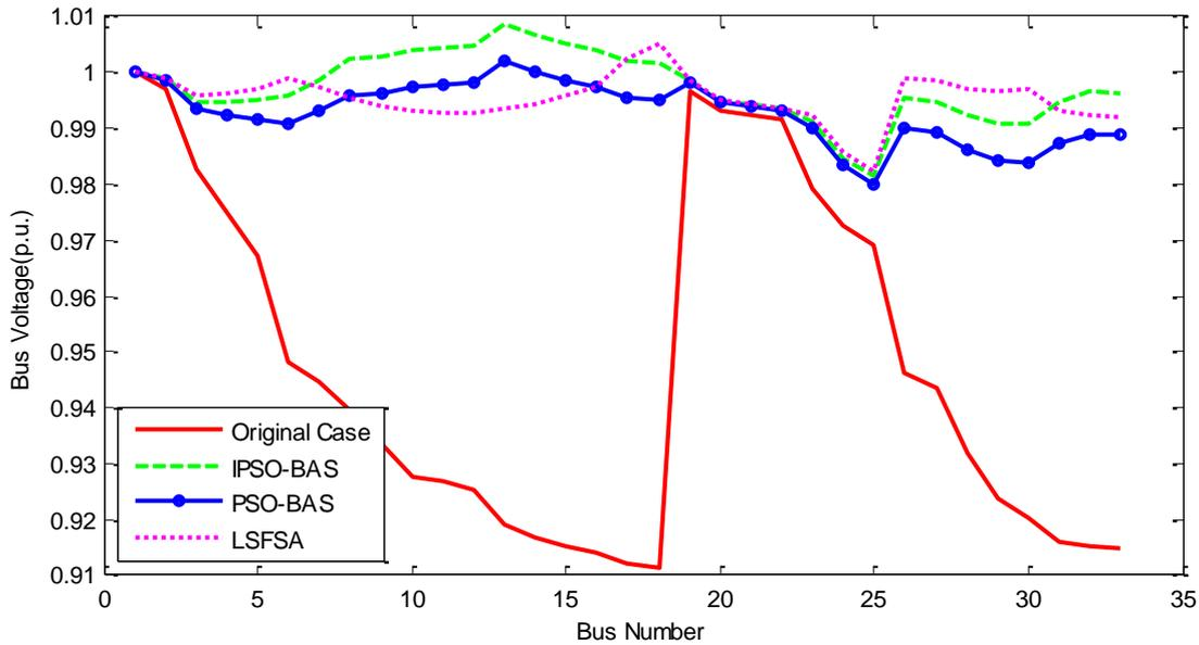
Fig.13 The node voltages for different algorithms and origin case on the IEEE 33-bus distribution network (0.866 leading power factor)
