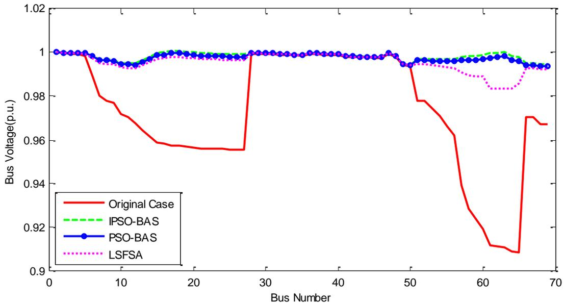
Fig.28 The node voltages for different algorithms and origin case on the IEEE 69-bus distribution network (0.866 leading power factor)
