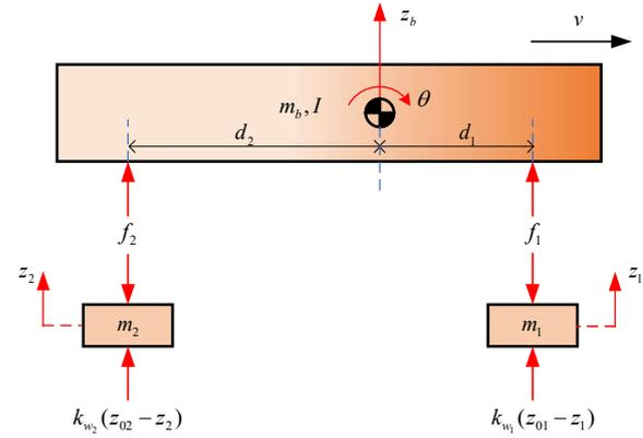
Fig. 2. Free body diagram of the half-car suspension model.
