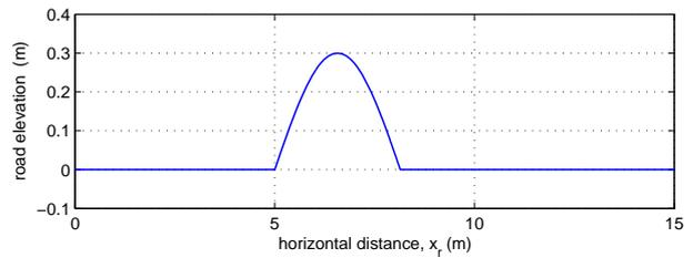
Fig. 3. Road profile and the road disturbance on both vehicle wheels.
