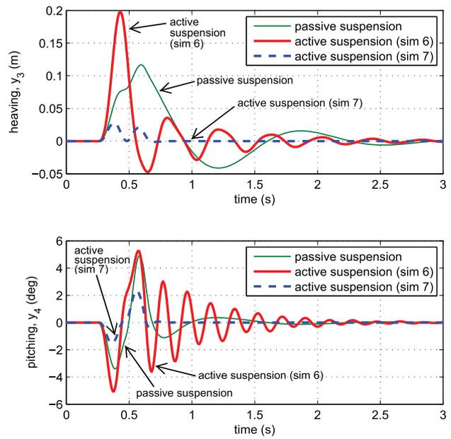
Fig. 6. The vehicle body motions of using passive and active suspension systems.
