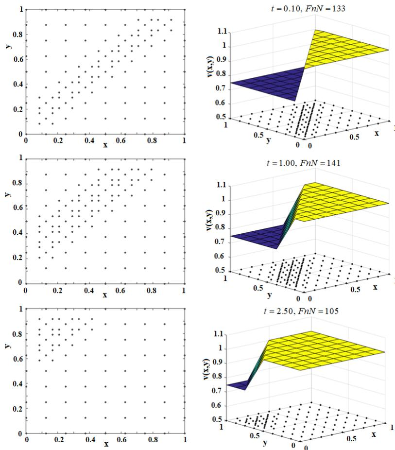
Fig. 7. Node distributions (left) with their corresponding solution profile (right) for V-velocity component numerically produced at  $Re = 1200$  with  $InN = 9 \times 9$ ,  $(\theta_{low}, \theta_{up}) = (0.25, 0.40)$  and  $\Delta t = 0.005$  measured at  $t = 0.1, 1.0$  and  $2.5$  respectively.
