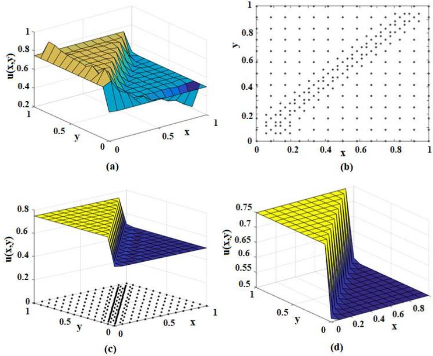
Fig. 5. Numerical simulation of U-velocity component at  $Re = 1,000$  with  $InN = 13 \times 13$  where (a) *DRBEM*, (b) Node distribution for *Adp-DRBEM*, (c) Improved solution profile, and (d) Exact surface.
