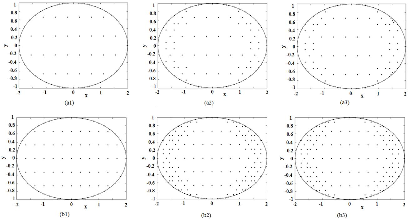
Fig. 2. Node distribution after undergoing the adaptation algorithm with 1- and 2- level of refinement where (a-) starting with  $InN = 68$  , and (b-) starting with  $InN = 91$ .
