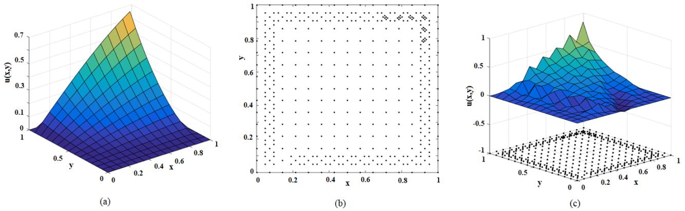
Fig. 4. Solution profiles at  $\gamma=1.00E-04$ ; (a) The exact profile, (b) Node distribution after undergoing the node-adaptation process with  $(\theta_{low}, \theta_{up})=(0.25,0.45)$ ,  $InN=225$ ,  $\epsilon_{MQ}=50$ , and (c) Numerical solution profile with its corresponding node-distribution with  $FnN=443$ .
