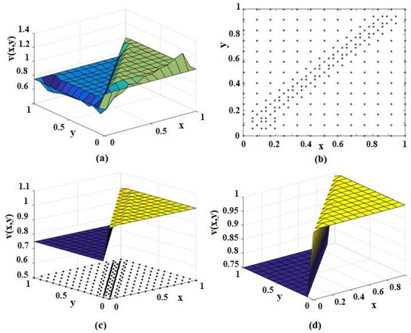
Fig. 6. Numerical simulation of V-velocity component at  $Re = 1,000$  with  $InN = 13 \times 13$  where (a) DRBEM, (b) Node distribution for Adp-DRBEM, (c) Improved solution profile, and (d) Exact surface.
