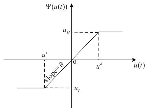
**Figure 1.** A typical nonlinear saturation function
