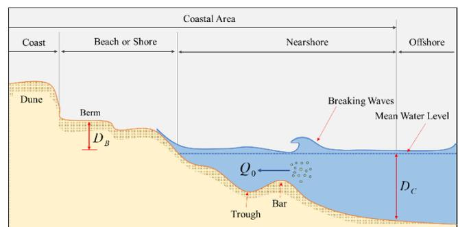
Fig. 4. Beach profile and shoreline physical parameters.
