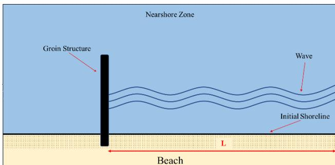
Fig. 1. Initial shoreline with configuration straight impermeable groins.
