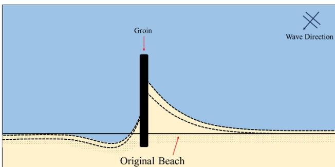
Fig. 2. Shoreline evolution with a groin structure.
