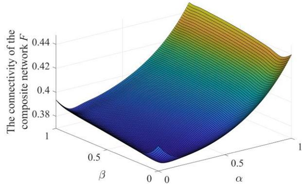
Fig.11 Graph of the effect of  $\alpha$  and  $\beta$  on the connectivity of the composite network
