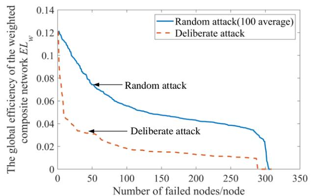
Fig.6 The global efficiency change diagram of the weighted composite network
