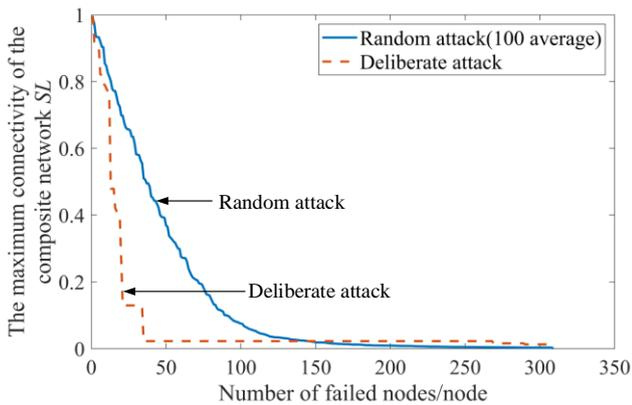
Fig.7 The maximum connectivity change diagram of the composite network
