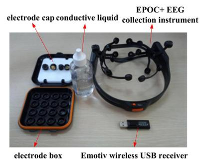
Fig. 7. EPOC+ EEG acquisition instrument
