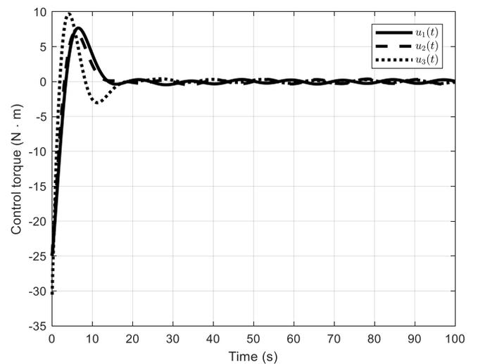
Fig. 5. Control torques of  $H_\infty$  controller at input saturation  $u_{\max} = 100$  and rate saturation  $v_{\max} = 100$
