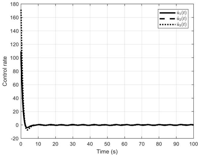
Fig. 11. Control rates of  $H_\infty$  controller at input saturation  $u_{\max} = 500$  and rate saturation  $v_{\max} = 500$
