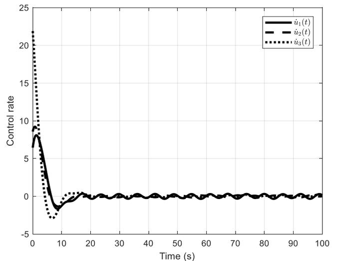
Fig. 6. Control rates of  $H_\infty$  controller at input saturation  $u_{\max} = 100$  and rate saturation  $v_{\max} = 100$
