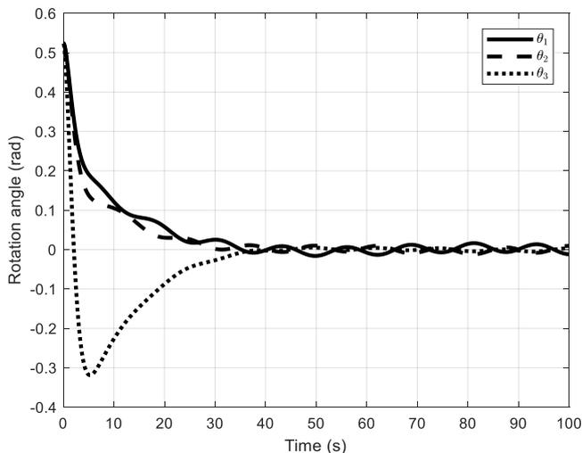
Fig. 7. Trajectories of rotation angles using  $H_\infty$  controller at input saturation  $u_{\max} = 500$  and rate saturation  $v_{\max} = 500$
