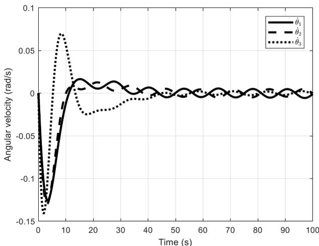
Fig. 3. Trajectories of angular velocity using the  $H_\infty$  controller at input saturation  $u_{\max} = 100$  and rate saturation  $v_{\max} = 100$
