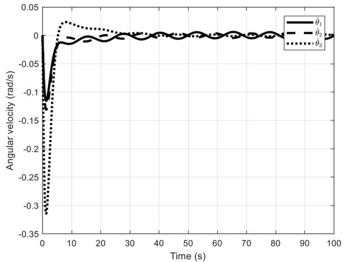
Fig. 8. Trajectories of angular velocity using  $H_\infty$  controller at input saturation  $u_{\max} = 500$  and rate saturation  $v_{\max} = 500$
