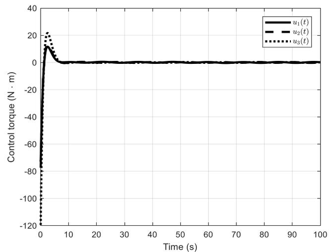
Fig. 10. Control torques of  $H_\infty$  controller at input saturation  $u_{\max} = 500$  and rate saturation  $v_{\max} = 500$
