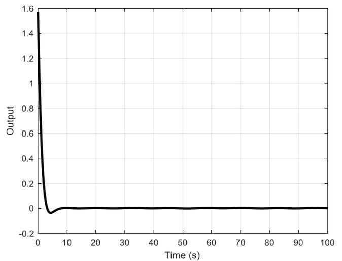
Fig. 9. Trajectory of output using  $H_\infty$  controller at input saturation  $u_{\max} = 500$  and rate saturation  $v_{\max} = 500$
