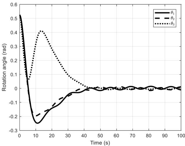
Fig. 2. Trajectories of rotation angles using the  $H_\infty$  controller at input saturation  $u_{\max} = 100$  and rate saturation  $v_{\max} = 100$
