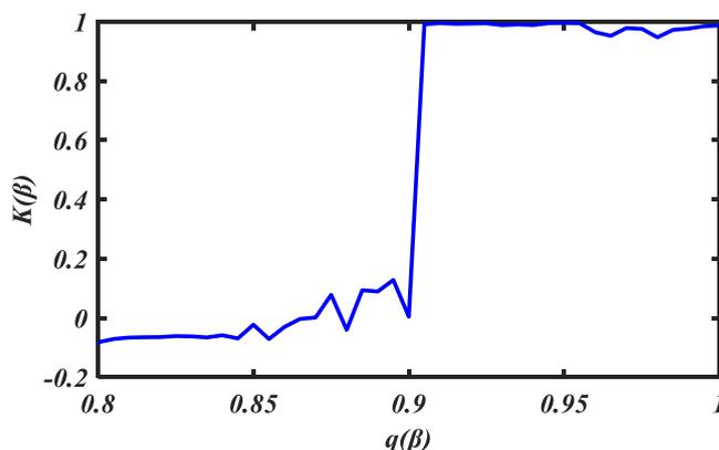
Fig. 9. The order  $K$  value diagram in accordance with the fractional-order chaotic system:  $q(\beta)$ - $K(\beta)$
