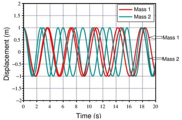
Fig. 2. Simple Harmonic Motion for Spring - Mass System under interval uncertainty with same amplitude
