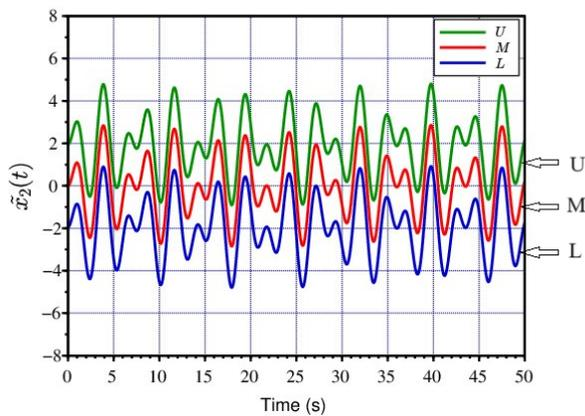
Fig. 5. Response of  $\tilde{x}_2(t)$  in Spring - Mass System with interval uncertainty
