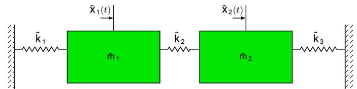
Fig. 1. Spring Mass System under interval uncertainty
