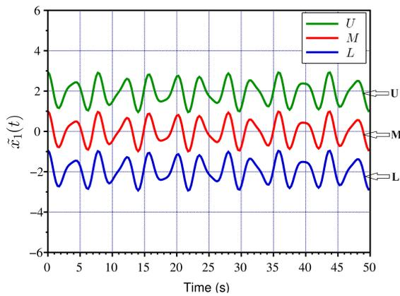
Fig. 4. Response of  $\tilde{x}_1(t)$  in Spring - Mass System with interval uncertainty
