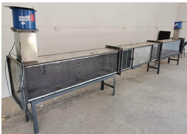
Fig. 1. Physical model of cable tunnel
