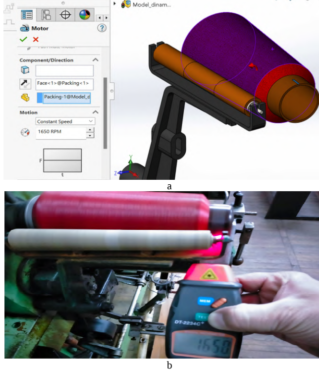
Fig. 4. Kinematic parameters of the winding mechanism: a - setting the parameters of the spool speed and direction from the computer model of the mechanism; b - indicators of the operating speed on the "Polycon" machine
