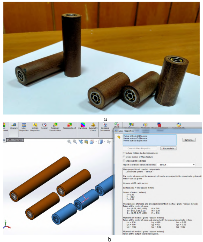
Fig. 3 Design of the roller: a - physical models of the elements of the rollers; b - computer solid models of the elements of the rollers and their mass-inertial parameters
