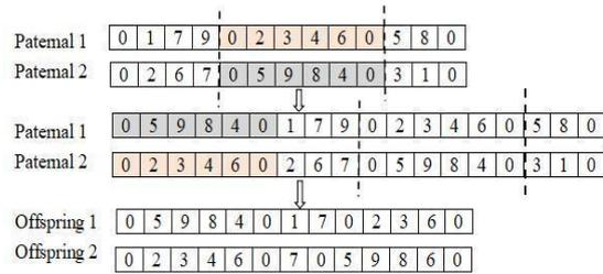
Fig. 2. Schematic diagram of the step-crossover operator
