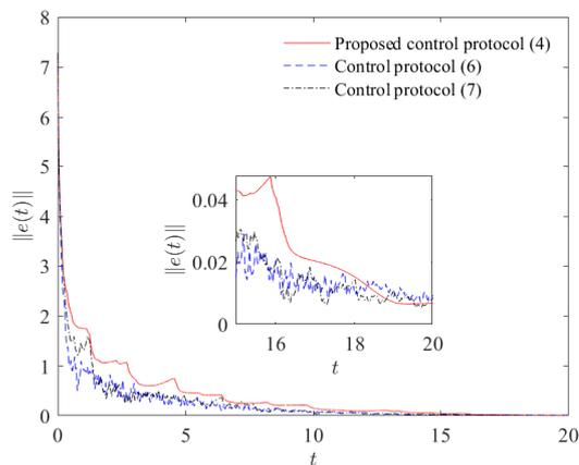
Fig. 8. The errors  $\|e(t)\|$  under different control protocols.
