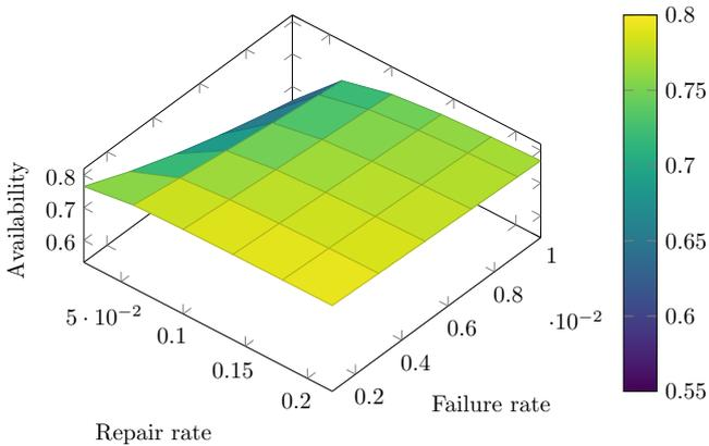
Fig. 5. Effect of Failure and Repair Rates of 'Jaw Crusher' Subsystem on Rock Gold Plant Performance
