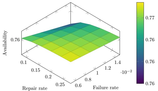
Fig. 9. Effect of Failure and Repair Rates of 'Shaking Table' Subsystem on Rock Gold Plant Performance
