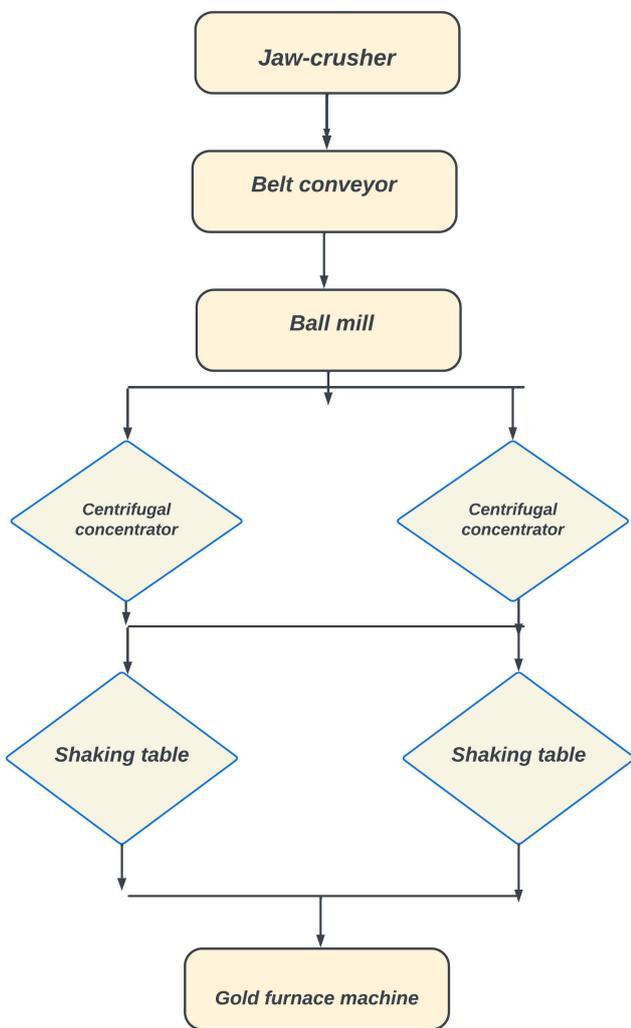
Fig. 2. Flow Diagram of Rock Gold Processing Plant
