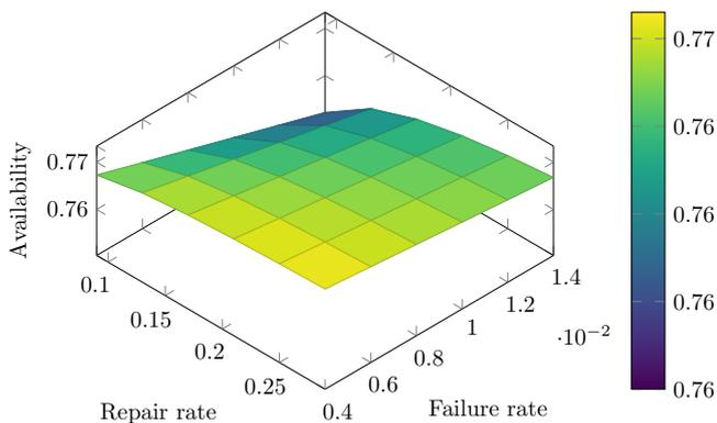
Fig. 8. Effect of Failure and Repair Rates of 'Centrifugal Concentrator' Subsystem on Rock Gold Plant Performance
