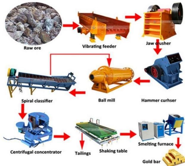
Fig. 1. Diagram of Rock Gold Processing Plant
