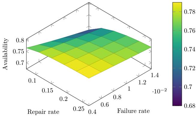
Fig. 7. Effect of Failure and Repair Rates of 'BALL MILL' Subsystem on Rock Gold Plant Performance
