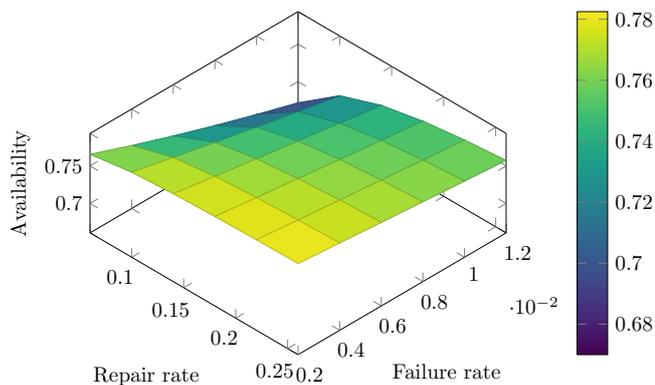
Fig. 10. Effect of Failure and Repair Rates of 'Gold Furnace Machine' Subsystem on Rock Gold Plant Performance
