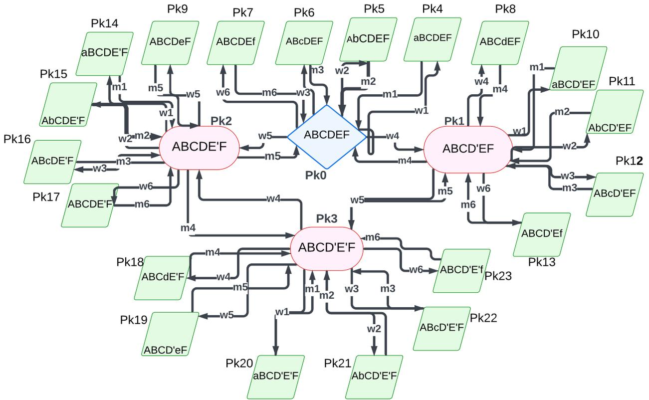
Fig. 3. Transition Diagram of Rock Gold Processing Plant
