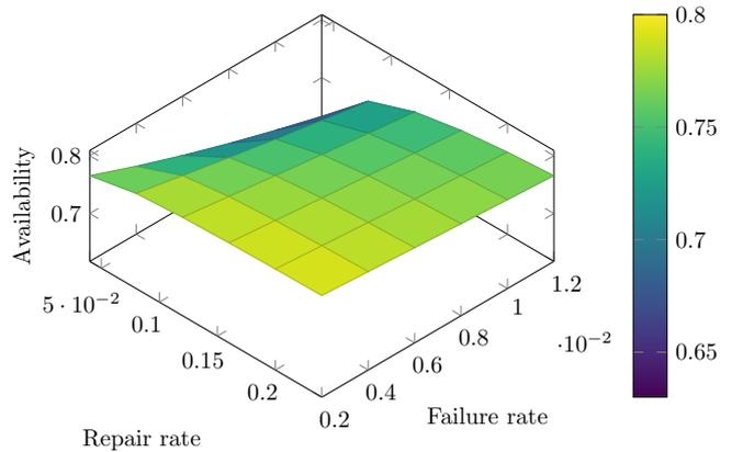
Fig. 6. Effect of Failure and Repair Rates of 'Belt Conveyor' Subsystem on Rock Gold Plant Performance
