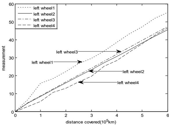
Fig. 2. The degradation paths of the left wheel
