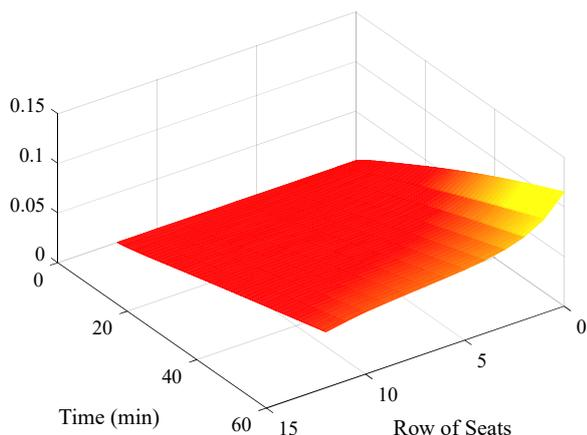
Fig. 3. The probability of airborne infection risk for susceptible individuals. Used the Forward-Time Centered-Space finite difference method.
