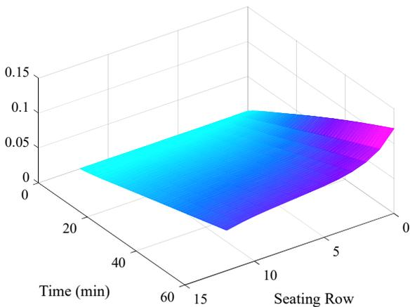
Fig. 10. The number of airborne infectious particles where  $\Delta t = 0.1$  and  $T = 60$ . Used the Crank-Nicolson implicit method.
