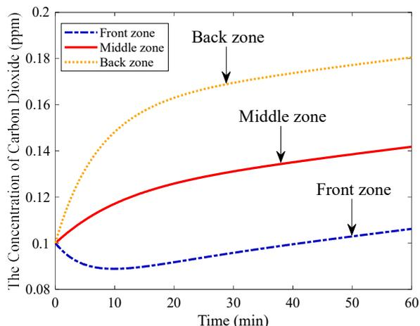
Fig. 6. The concentration of carbon dioxide in the air in the front, middle, and back zones on a bus with a ventilation system where  $\Delta t = 0.1$  and  $T = 60$ . Used the Crank-Nicolson implicit method.
