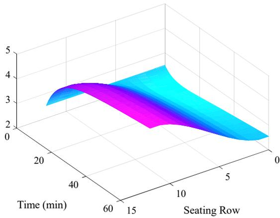
Fig. 8. The volume fraction of exhaled air on a bus where  $\Delta t = 0.1$  and  $T = 60$ . Used the Crank-Nicolson implicit method.
