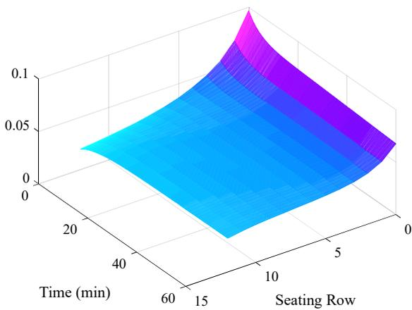
Fig. 9. The concentration of airborne infectious particles where  $\Delta t = 0.1$  and  $T = 60$ . Used the Crank-Nicolson implicit method.
