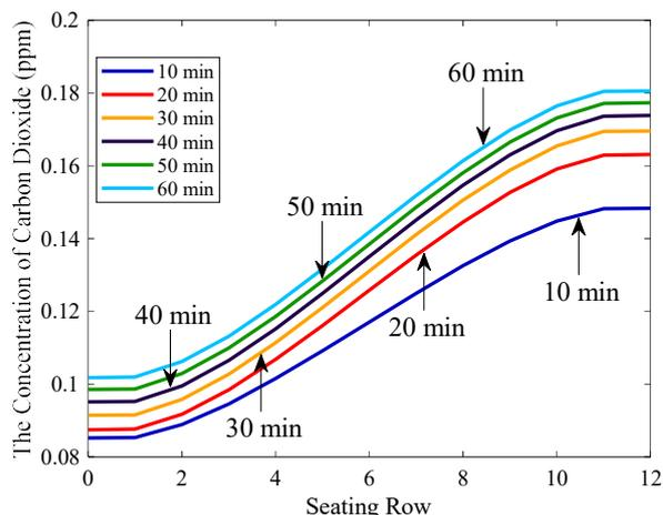
Fig. 7. The concentration of carbon dioxide in the air on a bus every 10 minutes with a ventilation system where  $\Delta t = 0.1$  and  $T = 60$ . Used the Crank-Nicolson implicit method.
