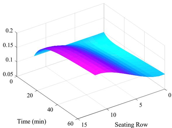
Fig. 5. The approximated carbon dioxide concentration in the air on a bus with a ventilation system where  $\Delta t = 0.1$  and  $T = 60$ . Used the Crank-Nicolson implicit method.
