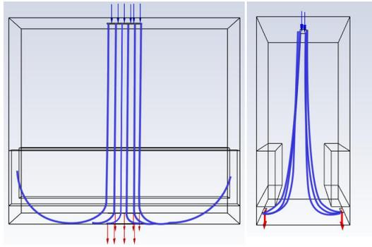
Fig. 11. Airflow field for a split air inlet.
