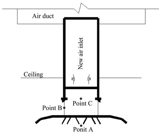
Fig. 8. Measuring point location.
