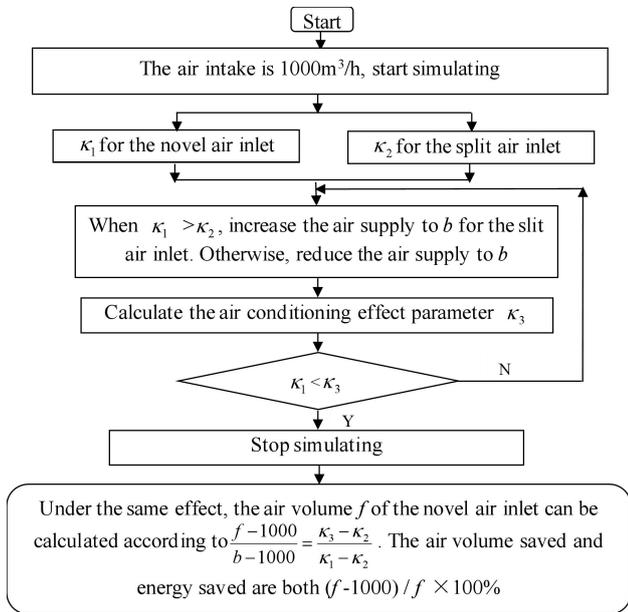
Fig. 12. The energy-saving calculation process for the novel air inlet.
