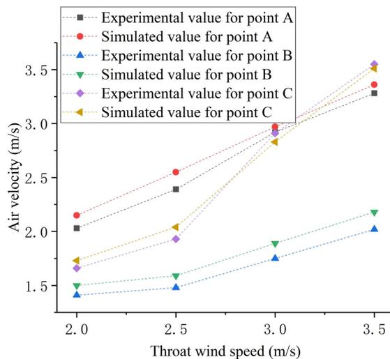
Fig. 9. Comparison of experimental values and CFD.
