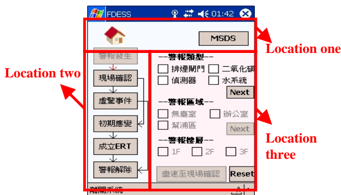
Fig. 7. The first fire control procedure of the FDESS (Fire Alarm)
