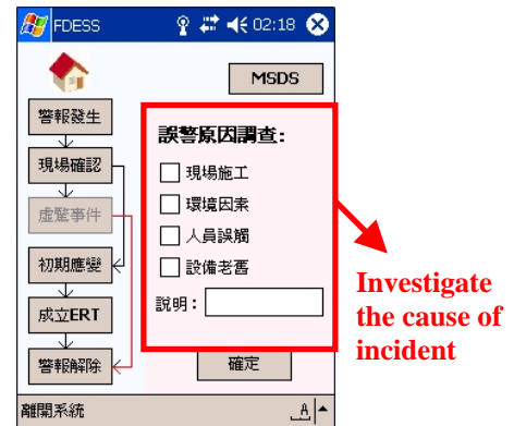
Fig. 9. The third fire control procedure of the FDESS (Incident Event)
