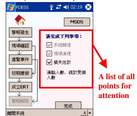
Fig. 12. The final fire control procedure of the FDESS (Recover System)
