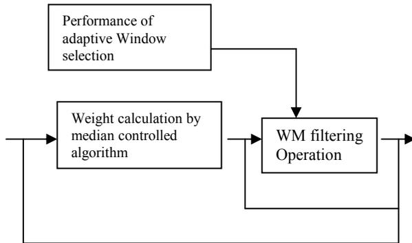
Fig1. Block diagram of Median controlled adaptive RWM filter
