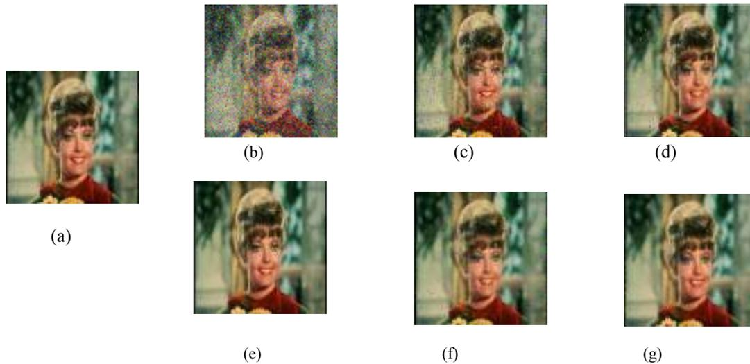
Fig 4. (a) Original Zelda 256 X 256 image (b) Noisy image (density 20%) (c) SMF outputs (d) WMF output (e) RWM output (f) MC LIN's output (g) Proposed ARWMF output
