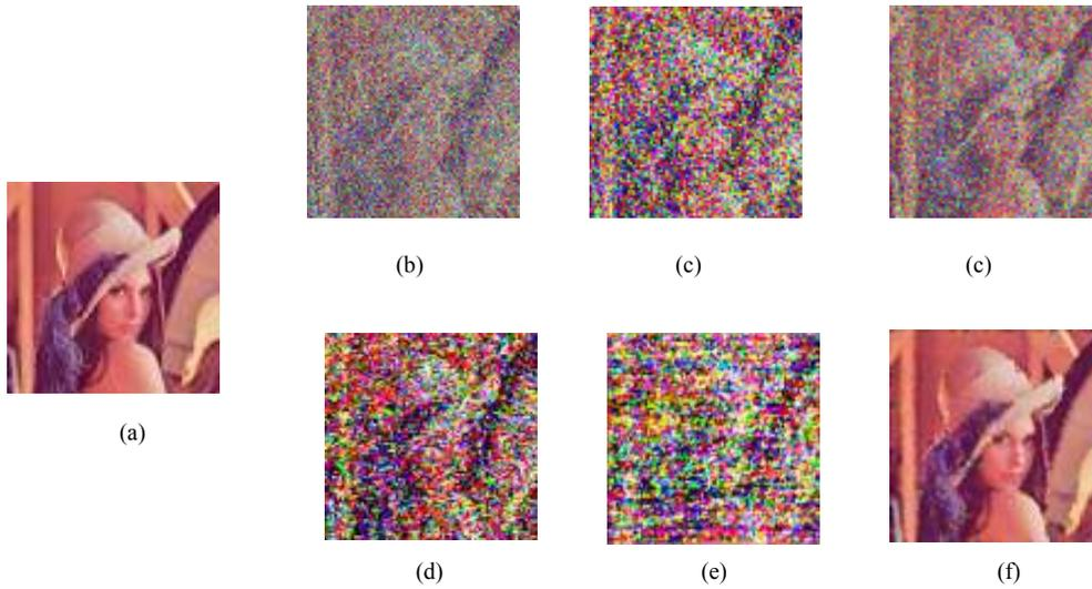
Fig 3. (a) Original Lena 256 X256 image (b) Noisy image (density 80%) (c) SMF outputs (d) WMF output (e) RWM output (f) MC LIN's output (g) Proposed ARWMF output
