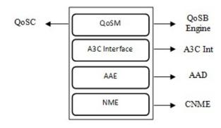
Fig. 5. The Access Router Structure
