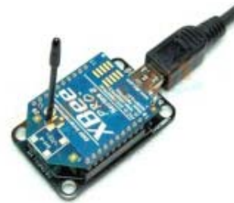
Figure 7. The xBee wireless component serving as the coordinator
