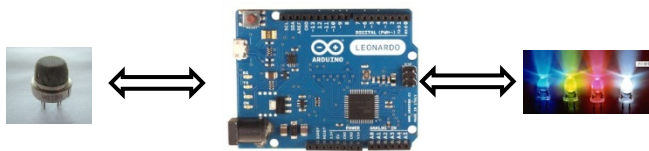
Figure 9. The traffic of data and the components involved in the process: (left) a sensor; (center) the Arduino board; (right) the LED lights. The arrows indicate the flow of information between the components.
