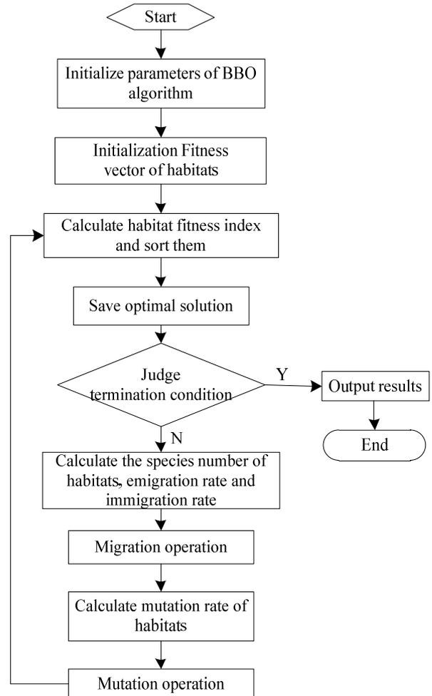
Fig. 5 Flowchart of Biogeography-Based Optimization algorithm.
