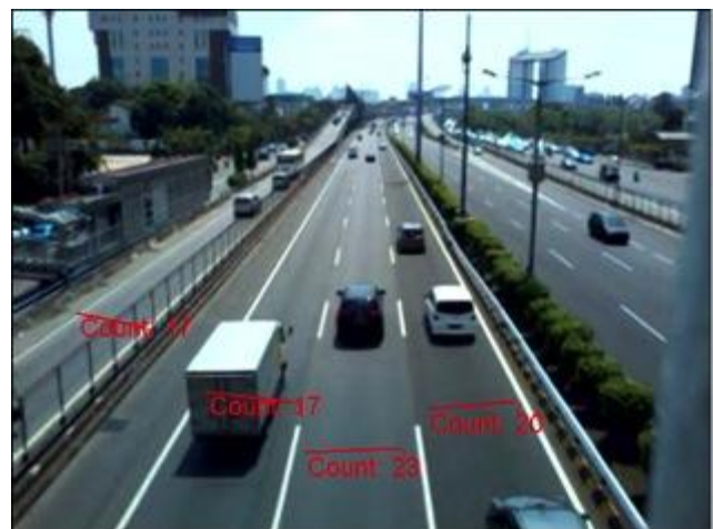
Fig. 17. Experimental result's screen capture of the object counting processes in daylight – on a road with lanes.
