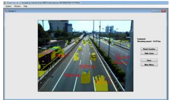
Fig. 11. Working application of moving object counters implementation on traffic flow. The shading overlaying every moving object (cars) on the screen is the marking created by the algorithms to show significant difference of the object pixels values and the background values. If the value of this pixel differences is larger than a certain value of granularity (threshold T ) then the count for that line is increased (marked with message: "Count: [numbers]").
