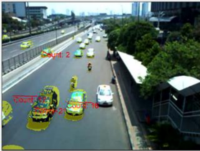
Fig. 12. Experimental result's screen capture of the object counting processes in daylight – no lane. The system could also record movement of motorcycles, cyclists and pedestrians that passed.
