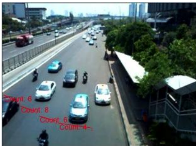
Fig. 15. Experimental result's screen capture of the object counting processes in daylight – four virtual lines on a road without lanes.
