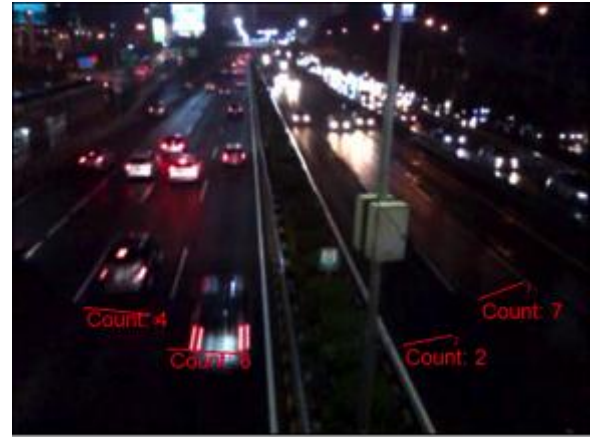
Fig. 19. Object counting processes at night using four virtual lines on road with lanes.
