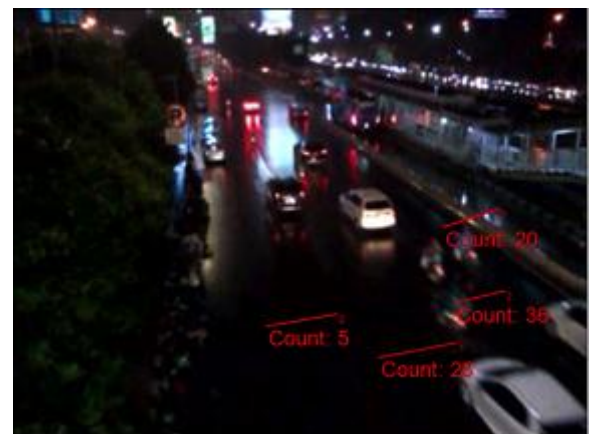
Fig. 21. Object counting processes at night using four virtual lines on a road without lanes.
