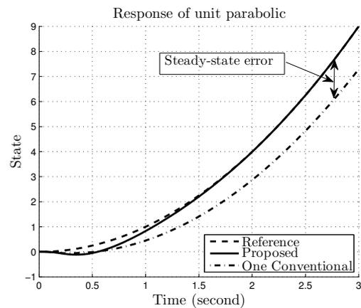
Fig. 10. Inverted pendulum response of unit-parabolic
