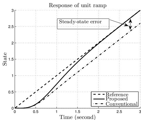
Fig. 7. DC motor response of unit-ramp
