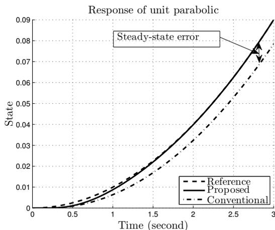
Fig. 8. DC motor response of unit-parabolic
