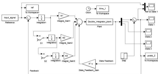
Fig. 13. Plant in simulink
