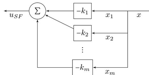
Fig. 3. The Block Diagram of State Feedback
