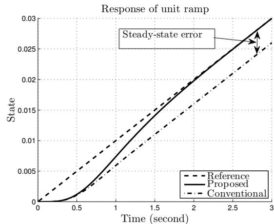
Fig. 5. Triple integrator response of unit-ramp
