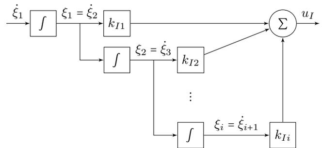
Fig. 2. The Block Diagram of  $n$ -Integrators
