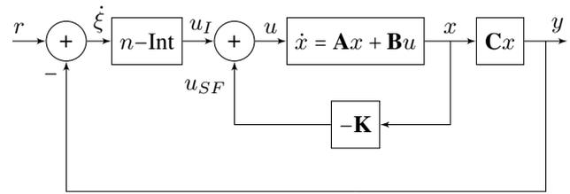
Fig. 1. The Block Diagram of Augmented System
