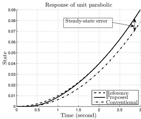
Fig. 6. Triple integrator response of unit-parabolic
