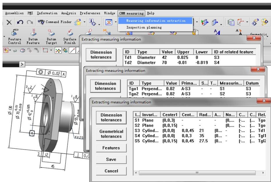
Fig. 8 Extraction of dimension tolerance, geometrical tolerance, and related features
