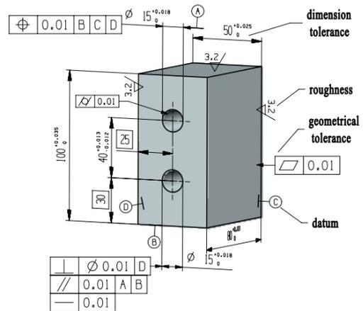
Fig. 1 MBD Dataset of a workpiece in UG NX
