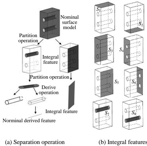
Fig. 5 The integral features and derived features of a nominal surface model
