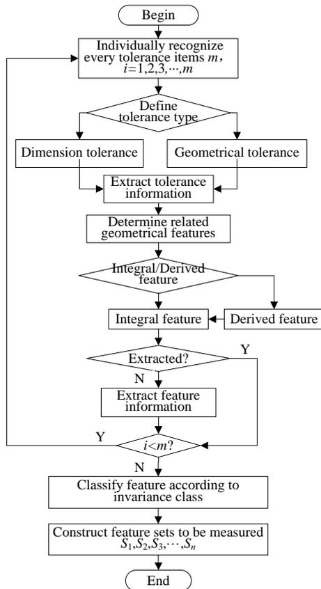
Fig. 7 The process of measuring information recognition and extraction
